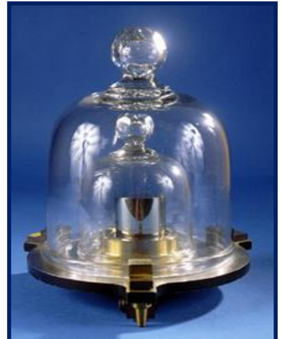
IPK, International Prototype Kilogram
