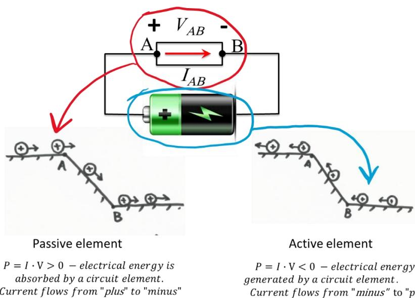
In case of a simple resistor we can use Ohm's law:  $U = I \cdot R$ , so the power is
