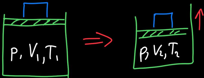
$$W_{\text{gas}} = p \cdot \Delta V = p \cdot (V_2 - V_1)$$
