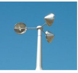
Wind speed is measured by anemometer (from Greek anemos 'wind').
