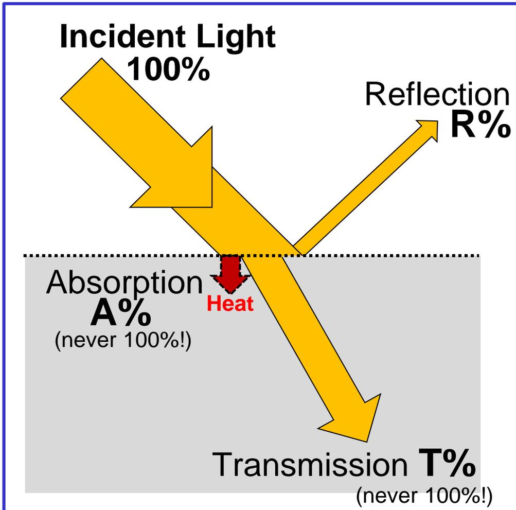
Light (energy!) can be **reflected**, **transmitted** or **absorbed** by matter.
