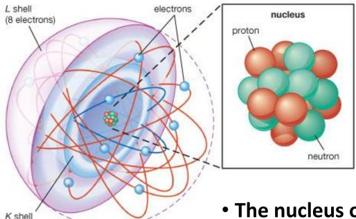
The <u>electrons</u> are kept in orbit around the nucleus due to an <u>electromagnetic field</u> of attraction between the positive (+) charge of the protons and the negative (-) charge of the electrons.
