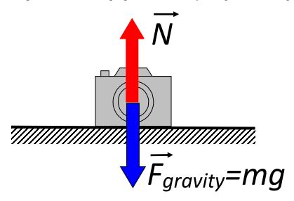
As we can see in the picture, if the camera just lies on the table, the magnitude of the normal force is equal to the magnitude of the gravity force.
