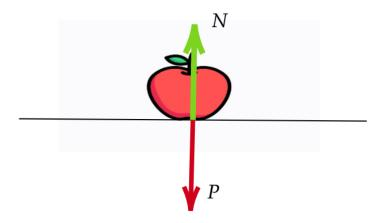
If an object is moving with acceleration, normal force (and therefore weight) change compared to when it is at rest. Let us assume that the same apple is in an elevator which is moving with acceleration a directed up. The net force up in terms of normal and gravitational forces is  $F_{net} = N - mg$ , and by Newton's second law for the apple:
