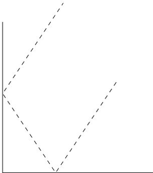
This property – or rather, similar property of corners in 3-D – is widely used: reflecting road signs (including stop signs), tail lights of a car, and reflecting strips on clothing are all constructed out of many small reflecting corners so that they reflect the light of a car headlamp exactly back to the car.
