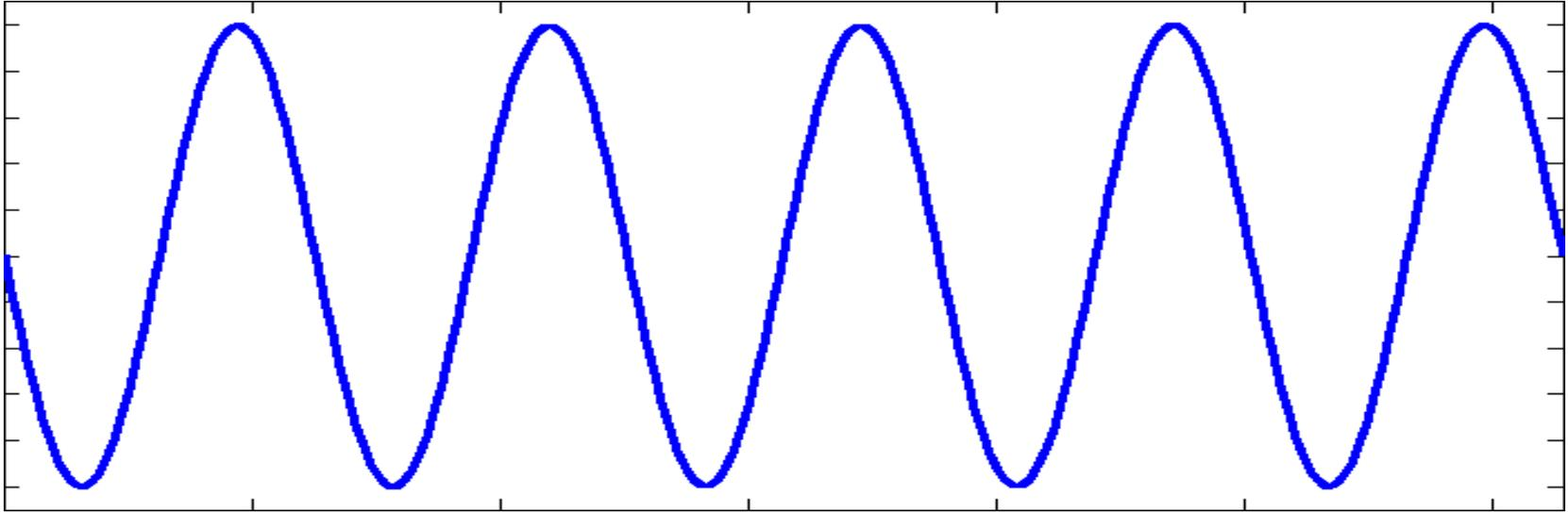
$$\text{FREQUENCY} = \frac{\text{VELOCITY (speed)}}{\text{WAVELENGTH}}$$
