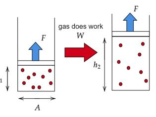
$$W = Fh = pA(h_2 - h_1) = p(Ah_2 - Ah_1) = p(V_2 - V_1) = p\Delta V.$$
