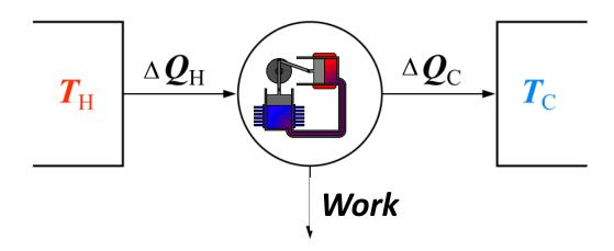
Heat Engine has to take heat  $\Delta Q_H$  from "heat bath", and return heat  $\Delta Q_C$  to a "cooler".
