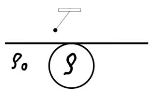
3. A uniform rod of mass *m* is connected to a slab as it is shown in the figure below. The force constant of the coil spring is *K*. The whole construction is placed on a frictionless table, so the table surface is parallel to the picture plane. The slab is attached to the table and cannot move. Find period of small oscillations of the rod. The moment of inertia of the rod with respect to the pivot point in the figure is  $ml^2/3$
