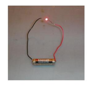
**Voltage** V is a potential energy of a unit charge. It tell you how much work the charge can do in an electric circuit. One typically measures a **Voltage difference** between two points in a circuit. It is similar to measuring height on a ski slope.
