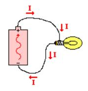
Electric current in the external circuit is directed from the positive to the negative terminal.
