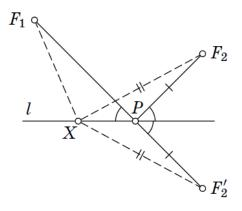
The interior and exterior points of an ellipse. The sum of the distances from any point inside the ellipse to the foci is less, and from any point outside the ellipse is greater, than the length of the major axis.
