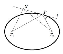
points of l the point P has the smallest sum of the distances to  $F_1$  and  $F_2$ . This means that the angles formed by the lines  $PF_1$  and  $PF_2$  with l are equal.
