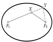
The optical property of the ellipse. A light ray passing through one focus of an elliptical mirror will pass through another focus upon reflection.
