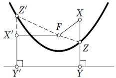
The optical property of the parabola. If a point light source, such as a small light bulb, is placed in the focus of a parabolic mirror, the reflected light forms plane-parallel beam perpendicular to the directrix (this is the principle used in spotlights). In other words, a light ray passing through one focus of a parabolic mirror upon reflection in such mirror will be perpendicular to the directrix of the parabola.
