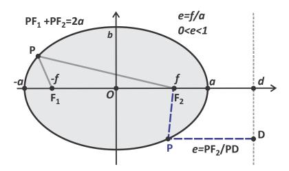
special points,  $F_1$  and  $F_2$  on the ellipse's major axis and are equidistant from the center point. The sum of the distances from point P on the ellipse to the foci is constant and equal to the major axis  $(PF_1 + PF_2 = 2a)$ .
