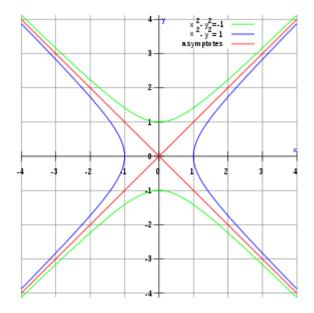
If b=a, the angle  $2\theta$  between the asymptotes equals  $90^\circ$  and the hyperbola is said to be rectangular or equilateral. In this special case, the rectangle joining the four points on the asymptotes directly above and below the vertices is a square, since the lengths of its sides 2a=2b.
