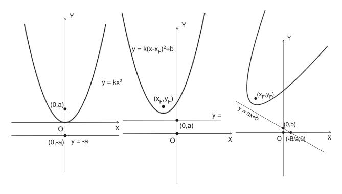
The easiest way to show that the above definition indeed corresponds to a parabola is by using the method of coordinates. Indeed, let line l be parallel to the X-axis and intersect the Y-axis at y = -a, and focus F(0, a) lie on the Y-axis at the same distance a from the origin. Then for any point on the parabola according to the definition above,
