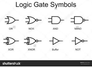
Combining such simple gates, one can create more complicated ones — and use that to create circuits which take as input a collection of binary digits and produce as output some function such as sum or product of inputs (interpeting n binary inputs as an n-digit binary number).
