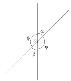
$\alpha$  and  $\beta$  and  $\phi$  and  $\psi$  are 2 pairs of vertical angles.
