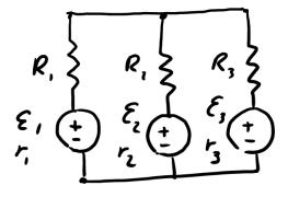
3. (more difficult) Current I in the circuit below is 1A, R=10 Ohm and internal resistances of the sources are 1 Ohm each. It was found that the magnitude of current I does not depend on resistance R1. Find e. m. f. of the sources (E<sub>1</sub> and E<sub>2</sub>).
