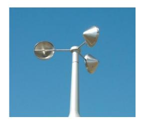
Wind speed is measured by anemometer (from Greek anemos 'wind').
