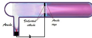
Figure 4: Anode tube. Anode rays are seen in the right part of the tube, behind the anode.
