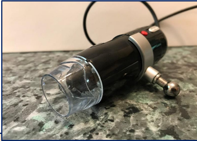
USB microscope, ~100X
