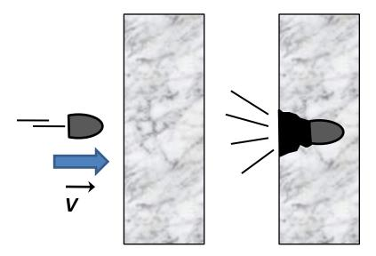
The bullet has relatively low mass (~10g) but it moves at a high velocity (~300-400m/s). We can calculate the momentum of the bullet: P=0.010kg.x 400m/s=4kgm/s. Imagine that the bullet hits a wall and stops in 0.01second. Let us calculate the force applied to the bullet by the wall (I choose the direction of the bullet motion as positive):
