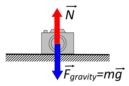
As we can see in the picture, if the camera just lays on the table, the magnitude of the normal force is equal to the magnitude of the gravity force. Choosing "up" as positive direction we have:
