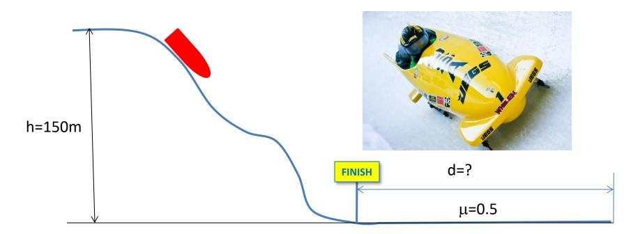
**Problem 2.** A bobsleigh goes down the track whose initial point is at height h=150 m. If there were no friction and no air resistance during the descend, find the distance d that bobsleigh had to travel after the finish line, before coming to a complete stop. Coefficient of kinetic friction on that horizontal part of the trip is  $\mu=0.5$ .
