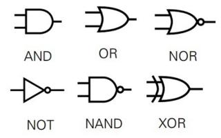
Combining such simple gates, one can create more complicated ones — and use that to create circuits which take as input a collection of binary digits and produce as output some function such as sum or product of inputs (interpreting n binary inputs as an n-digit binary number).
