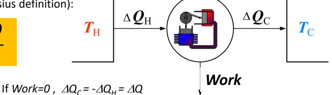
$$\Delta S_{total} = \frac{\Delta Q_C}{T_C} - \frac{\Delta Q_H}{T_H} = \Delta Q \left( \frac{1}{T_C} - \frac{1}{T_H} \right) \geq 0$$
