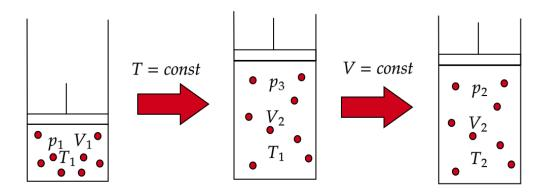
FIGURE 1. We could reach the final state  $p_2, V_2, T_2$  in two steps: first keep temperature constant and then keep volume constant.
