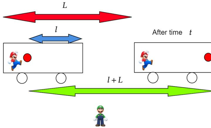
Distance  $l$  traveled by the ball in carriage reference frame is  $l = v_1 t$ . The carriage itself travels  $L = vt$ . So our friend outside sees the ball moving by  $l + L = v_1 t + vt = (v_1 + v)t$ . Now we could find the speed of the ball with respect to the outside observer :
