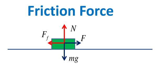
STATIC FRICTION Imagine that you try to move a block on a floor by pushing it with force F. The block does not move because of static friction with the floor. That force oppose motion, and will be equal to F to make sure that the block is at rest. However it cannot be bigger than certain maximum value:
