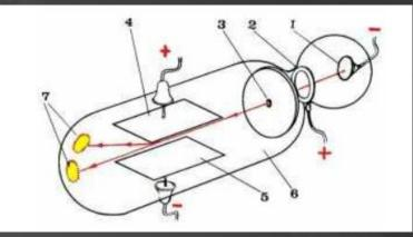
Thomson's cathode ray tube 1 – cathode; 2 – anode; 3 – hole; 4 and 5 – electrodes to bend the rays; 6 – phosphorescent coating, 7 – phosphorescent spots.
