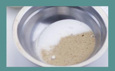
A <u>Mixture of Sand and Table Salt</u> can be separated according to solubility.
