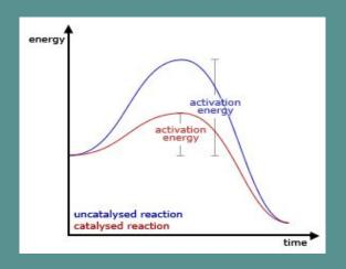
A catalyst works by providing an alternative activation pathway for the reaction to occur. This pathway has a lower activation energy than the pathway without the catalyst.
