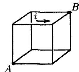
5. Each side of a circuit shown on the figure has the same resistance  $r$ . Find the total resistance between the points  $A$  and  $B$ ; between the points  $C$  and  $D$ .
