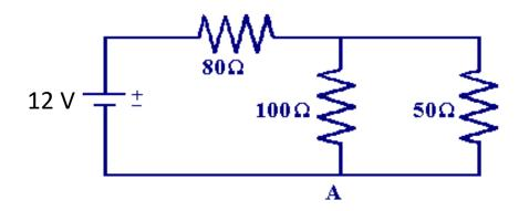
c) You need to replace one of the resistors in the circuit above with a light bulb, so that the current through the bulb were the smallest possible. Which one will you replace?
