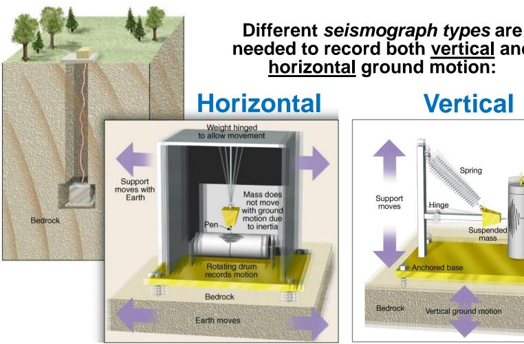
needed to record both vertical and horizontal ground motion:
