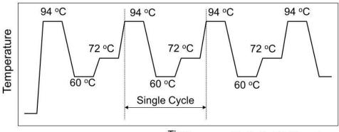
Time Typically 25-35 cycles performed during PCR
