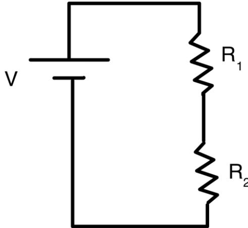
**Series:** The current flowing through  $R_1$  and  $R_2$  is the same, so
