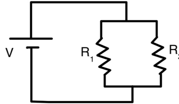
**Parallel:** The current splits between  $R_1$  and  $R_2$ , so
