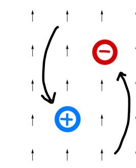
For a negative charge, the behavior changes. Moving it up increases its potential energy since the electric force pulls downwards.
