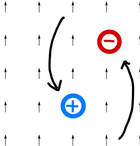
For a negative charge, the behavior changes. Moving it up increases its potential energy since the electric force pulls downwards.
