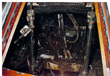
Figure 8: Apollo 1 cabin's interior after fire.
