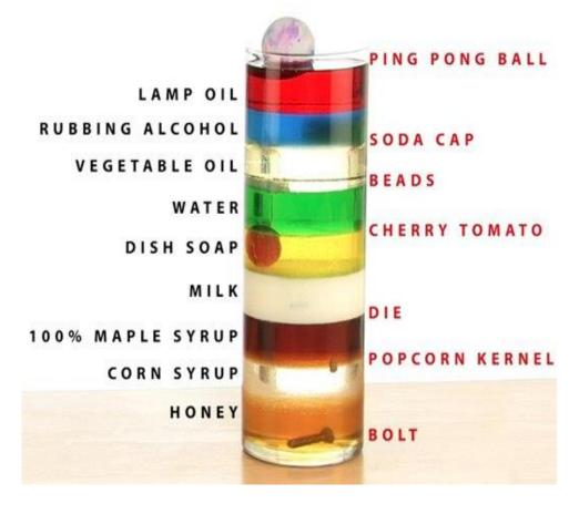
The term "miscibility" describes how well two substances mix. "Immiscible" liquids do not mix. When combined together, they form layers.
