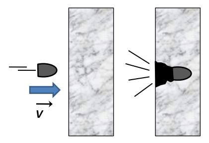
The bullet has relatively low mass (~10g) but it moves at a high velocity (~300-400m/s). We can calculate the momentum of the bullet: P=0.010kg.x 400m/s=4kgm/s. Imagine that the bullet hits a wall and stops in 0.01 second. Let us estimate the force applied to the bullet by the wall (I choose the direction of the bullet motion as positive):
