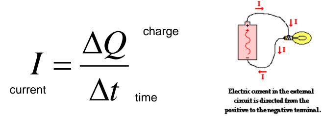
Electric Current (represented by letter I) is the total charge flowing through a wire in 1 sec. Measured in Amperes [A] (Coulomb per second) : 1A=1C/s.
