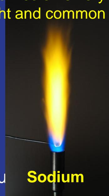
Many metals produce flame colors made by electrons jumping up to a higher orbit in the atom when it is heated, but they soon fall down, putting out light as energy.
