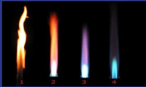
A flame test is a test for chemicals. Normally it is used to see certain metals in a chemical compound. This chemical compound is heated in a flame and a new colored flame is made. The colored flame can now be turned into a spectrum to be analyzed.
