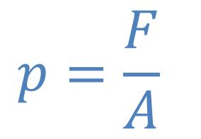
Unit of pressure is called pascal,  $1 \text{ Pa}=1 \text{N}/1 \text{m}^2$
