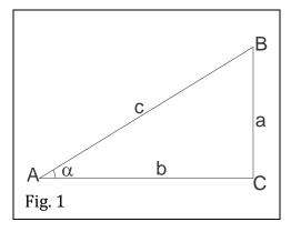
**Definition**. The <u>cosine</u> of  $\alpha$  is the ratio of the length of the leg adjacent to this angle to the length of the hypotenuse of the triangle.
