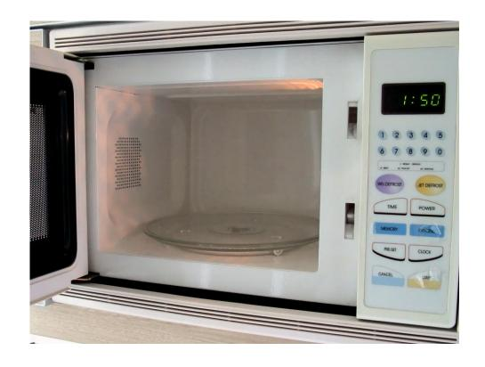
This is exactly what causes <a href="https://exactly.com/hot-spots">hot spots</a> and <a href="cold-spots">cold spots</a> in the food. The rotating turntable moves the food around to mitigate this effect.
