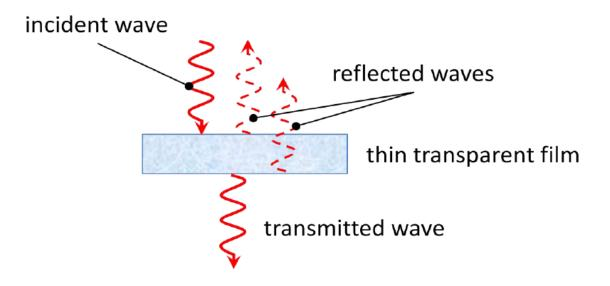
Figure 1. Interference in a thin film.
