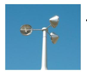
Wind speed is measured by anemometer (from Greek anemos 'wind').
